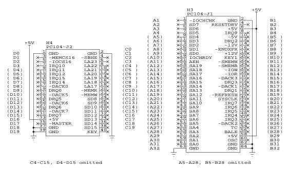
The MB implements a subset of the PC/104 specification in the form of two connectors that provide only +5V and GND for PC/104 modules. Only a total of 32 pins are implemented, 16 on J1 and 16 on J2. By adding up to four 8-pin connectors to the MB, PC/104 modules can be plugged directly into the MB to obtain +5V power and GND. No other connections between the PC/104 bus and the CubeSat Kit Bus are provided.
