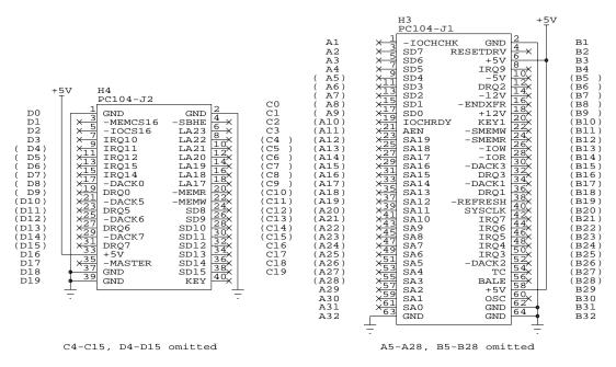
The DB implements a subset of the PC/104 specification in the form of two connectors that provide only +5V and GND for PC/104 modules. Only a total of 32 pins are implemented, 16 on J1 and 16 on J2. By adding up to four 8-pin connectors to the DB, PC/104 modules can be plugged directly into the DB to obtain +5V power and GND. No other connections between the PC/104 bus and the CubeSat Kit Bus are provided.
