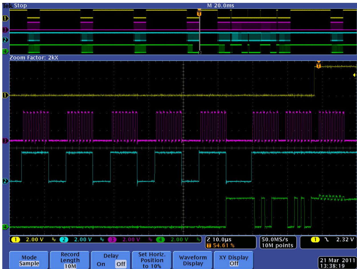
Figure 8: CubeSat Kit /8051 Rev D SD Card transfers at 1MHz
